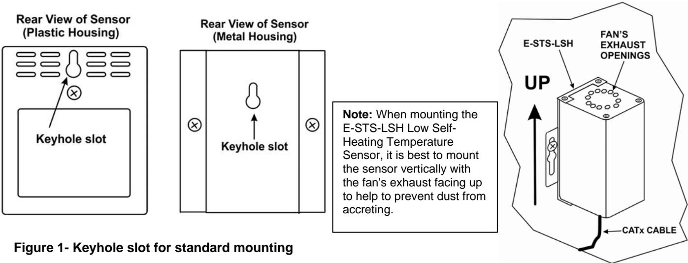
Figure 1- Keyhole slot for standard mounting
