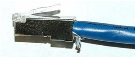
4. Set the RJ45 connector into the housing such that the snap handle is in the notch.
