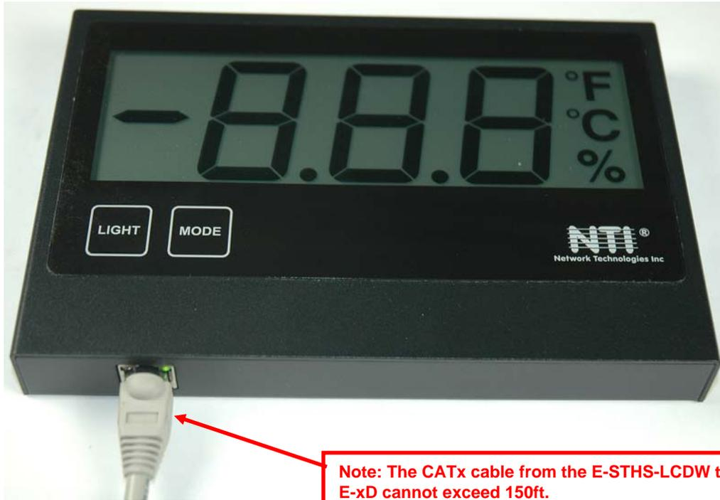
**Note: The CATx cable from the E-STHS-LCDW to the E-xD cannot exceed 150ft.
