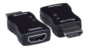
The HD4K-EDID-EMLTR HDMI 2.0 EDID Emulator copies the EDID of the desired HDMI display and connects directly to the HDMI source to ensure that the EDID is not lost in connections between devices such as switches, splitters, and extenders.
